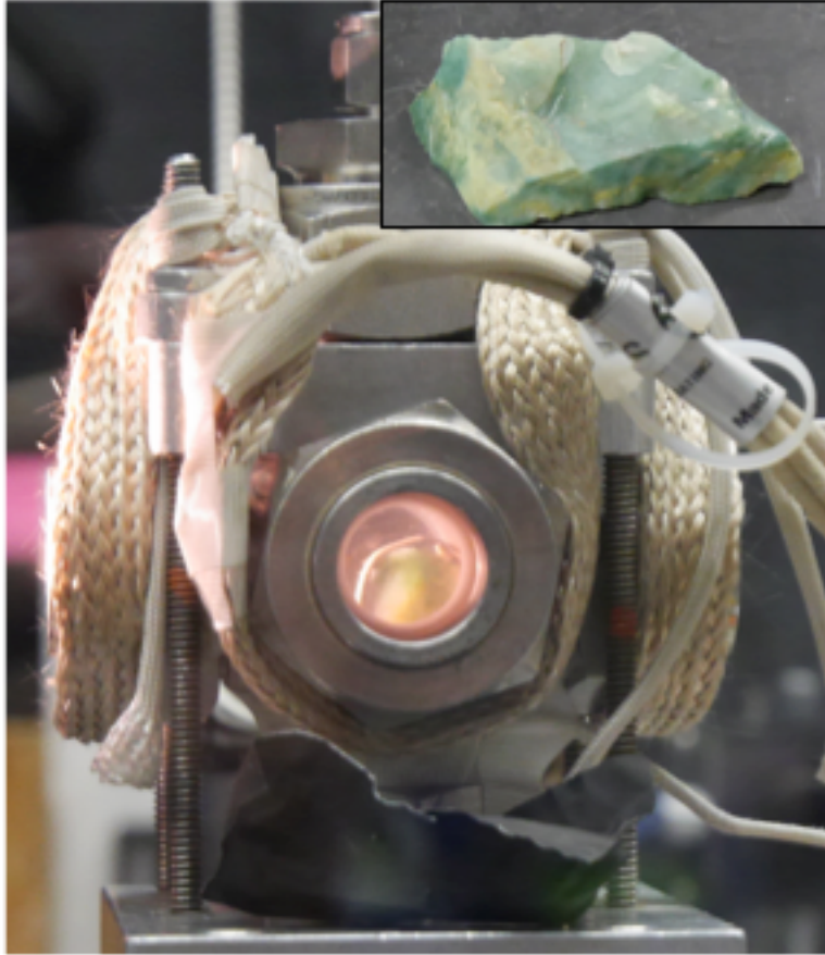
Figure 4.4. Supercritical CO 2 cell wrapped in heat tape with a piece of olivine held in the center.
